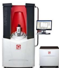
MPMS 3 SQUID MAGNETOMETER Temperature Range: 1.8K - 400K Magnetic Field: \pm 7 T
