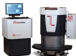
PPMS DYNACool (CRYOGEN FREE) Temperature Range: 1.8K - 400K Magnetic Field: \pm 14 T
